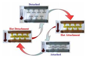
Figure 14. SMP fasteners' operation cycle
