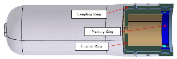
Figure 11. Test motor case with modified aft closure
