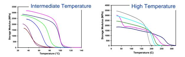
Figure 3. Examples of tailored SMP polymers in the expected range of useful activation temperatures for solid propellant rocket motors
