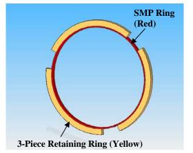
Figure 6. Retaining ring configuration
