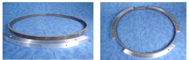
Figure 9. Attachment of SMP composite ring to three-piece metallic retaining ring
