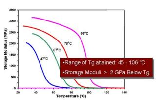
Figure 1. Veriflex elastic modulus versus temperature
