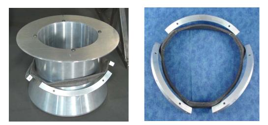
Figure 10. Released nozzle (left) and activated retaining ring (right)
