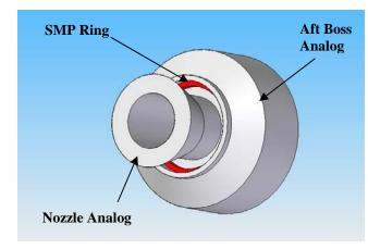
Figure 5. SMP internal retaining ring concept
