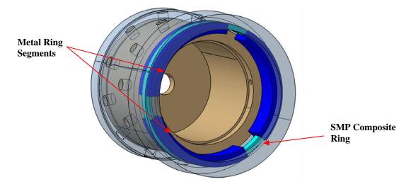
Figure 12. CRG's Phase II internal retaining ring design
